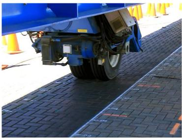
A Heavy Vehicle Similar applied up to 2.6 million ESALs on PICP section in dry and saturated conditions. The response of the pavement was used to calibrated models to determine the PICP subbase thickness.
