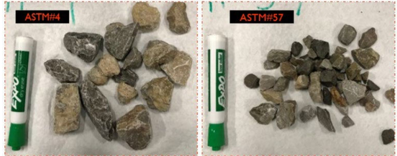
Photographs Showing Representative Particles from ASTM#4 and ASTM #57 Aggregate Materials
