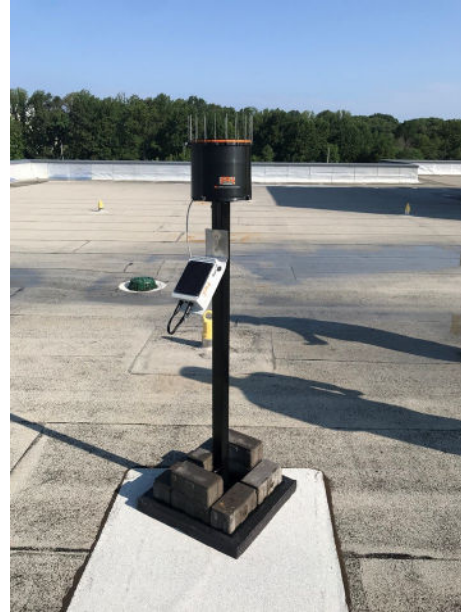
Figure 4: Rain gauge on ASCE headquarters rooftop.
