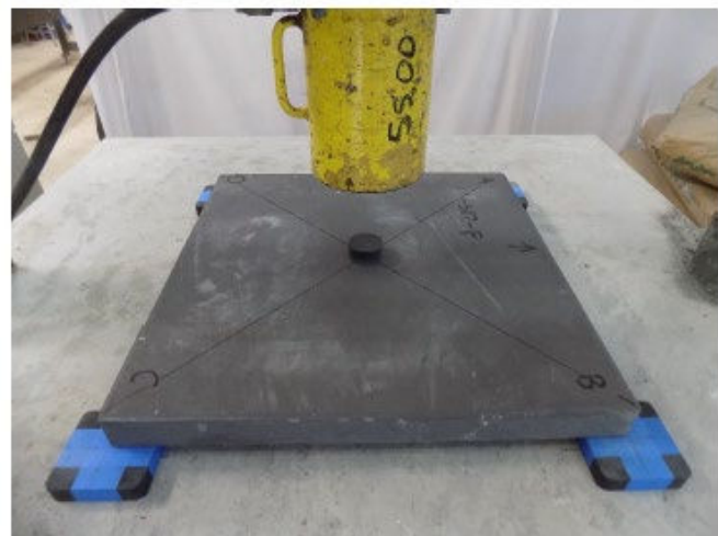
Figure 2: Corner Supported, Center Point Loading Testing Conditions
