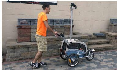
In 2018, Pathvu measured 96 various concrete permeable and non-permeable concrete paver surfaces in the Pittsburgh, Philadelphia/New Jersey, and Northern Virginia areas using their PathMeT device shown to the left. Data regarding joint width, chamfer width, imagery, and Wheelchair Pathway Roughness Index (WPRI) values were collected according to ASTM E3028. The results were compared against published suggested thresholds by Duvall for the U.S. Access Board which follow:
