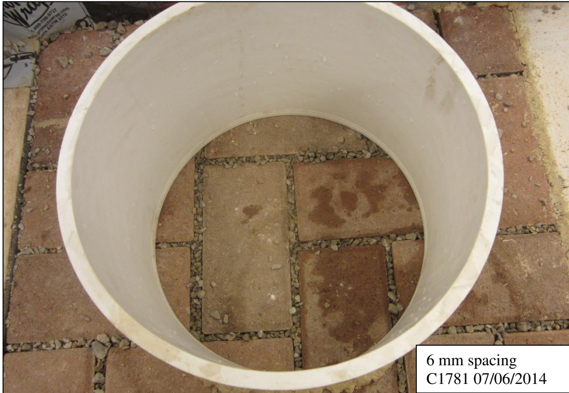
Figure 35. Vertical Infiltration C 1781 Test
