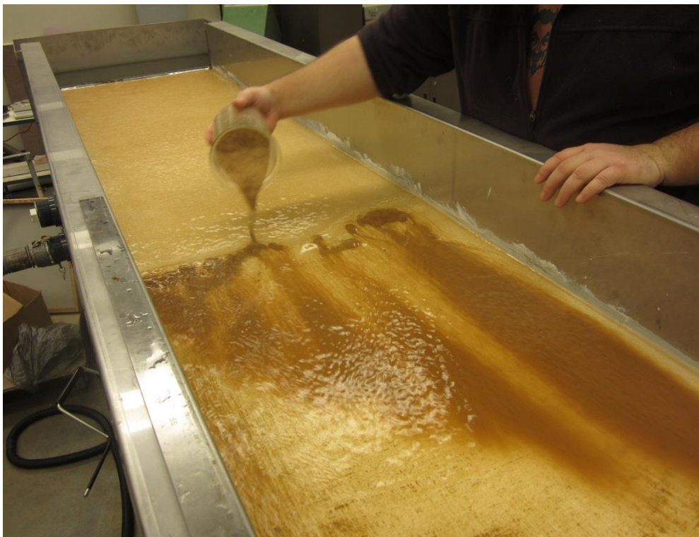
Figure 56. Synthetic Stormwater Dispensed Upstream of the Test Section
