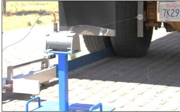
Figure 2.6: Encoder for measuring wheel location.
