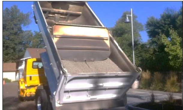
Figure 2.3: Re-distribution of aggregate to change load.
