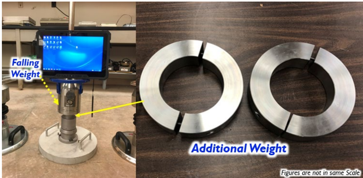
Figure 18: LWD Impact Compaction additional weights
