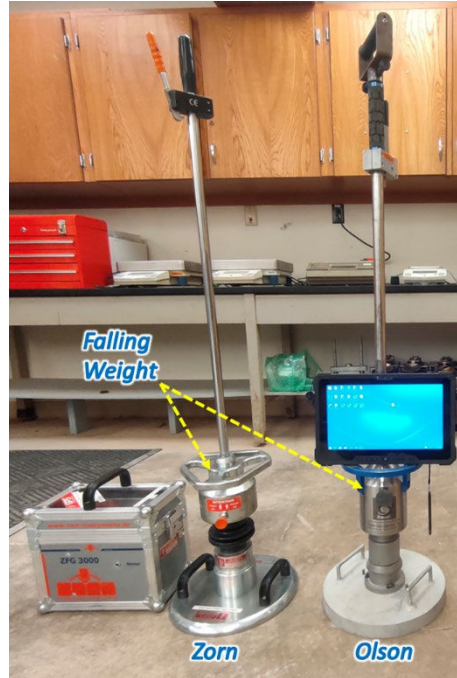
Figure 17: Photographs Showing the LWDs selected for Use in this Study: Zorn 3000 (Left), Olson (Right)
