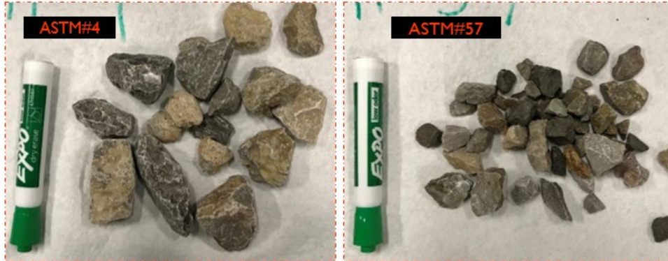
Figure 13: Photographs Showing Representative Particles from ASTM #4 and ASTM #57 Aggregate Materials
