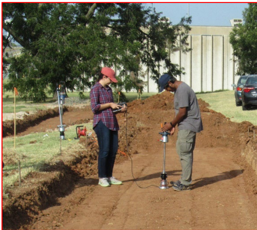
Zorn lab LWD Testing on Subgrade
