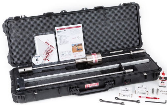
Figure 32: Photograph Showing the Dynamic Cone Penetrometer (DCP) with Accessories.
