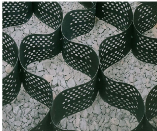
Figure 21: Photograph Showing a Geocell-Reinforced Aggregate Layer Constructed Inside the Wooden Box
