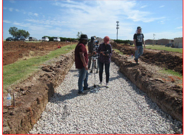
LWD Testing on 1 st Lift after Compaction
