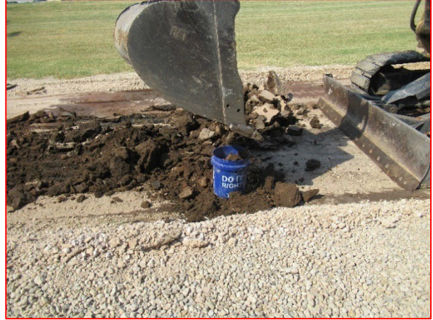
Soil Sample Collection for Laboratory Testing
