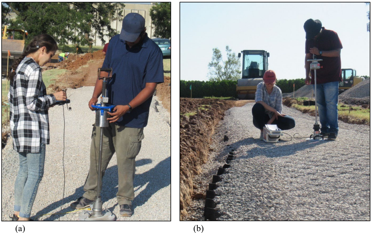
Figure 35: Photographs Showing LWD Testing on Aggregate Layers Placed in the Geocell-Reinforced Test Section: (a) Olson LWD-1; (b) Zorn ZFG-300
