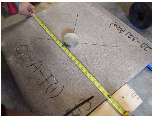
Figure 6 – Center Point Steel Loading Disk (Pilot Testing)
