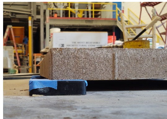
Figure 4 – Vulcanized Rubber Support Pads
