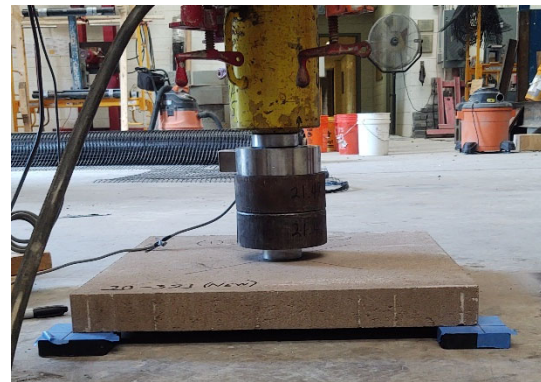
Figure 6 – Center Point Steel Loading Disk (Pilot Testing)
