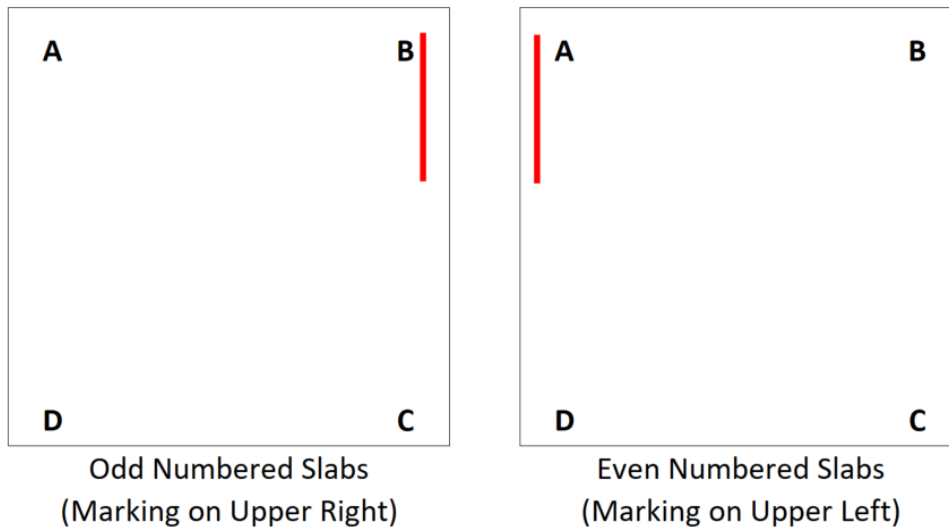
Figure 13 – Full-Size Slab Corner Markings
