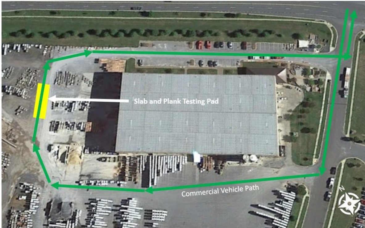
Figure 2: Nicolock’s Fredrick, Maryland plant - truck hauling route across test pad
