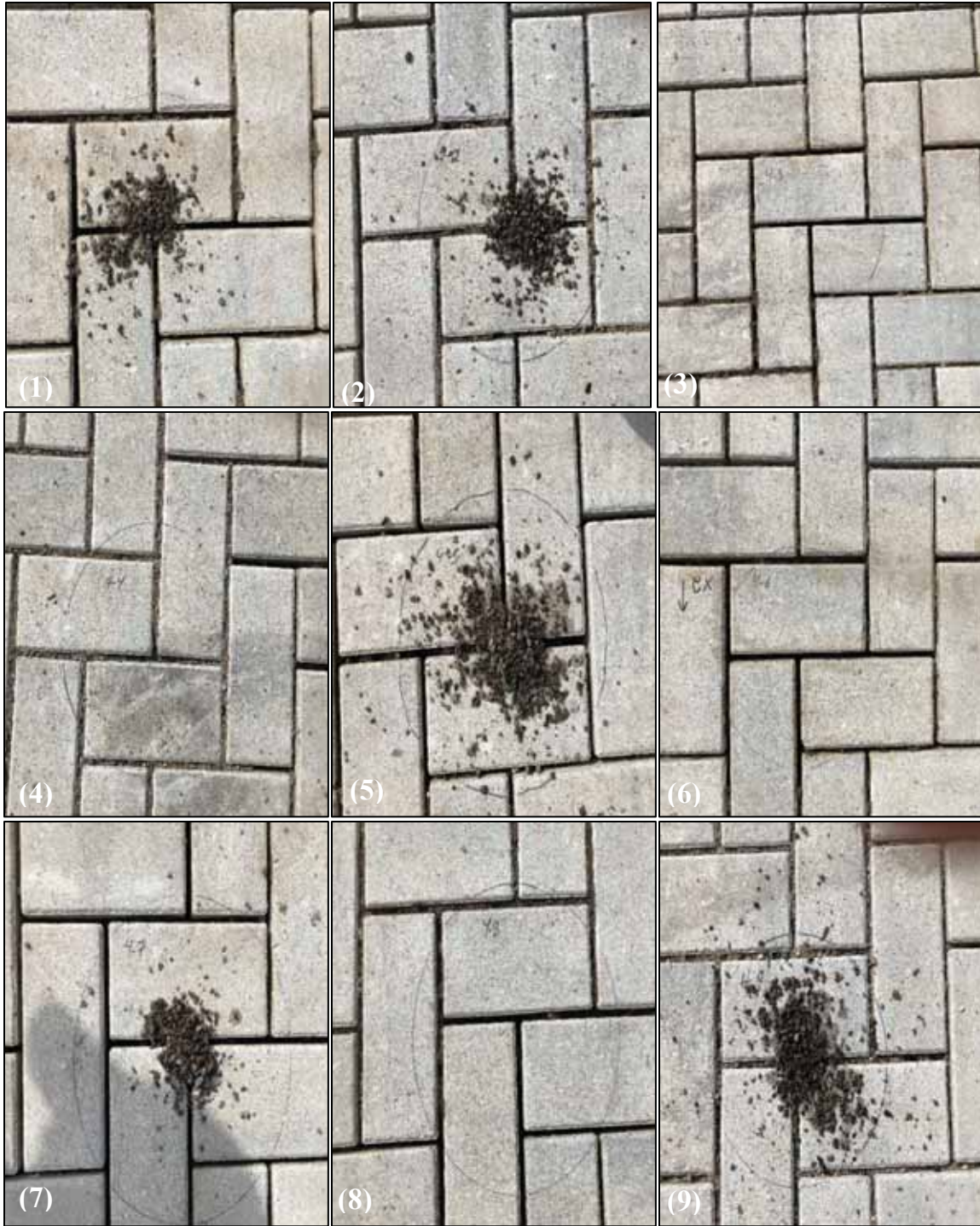
Figure 16. Post-maintenance photos of infiltration measurement locations (1-9) following a vacuum street sweeper on Cell 4 (Elgin Whirlwind).
