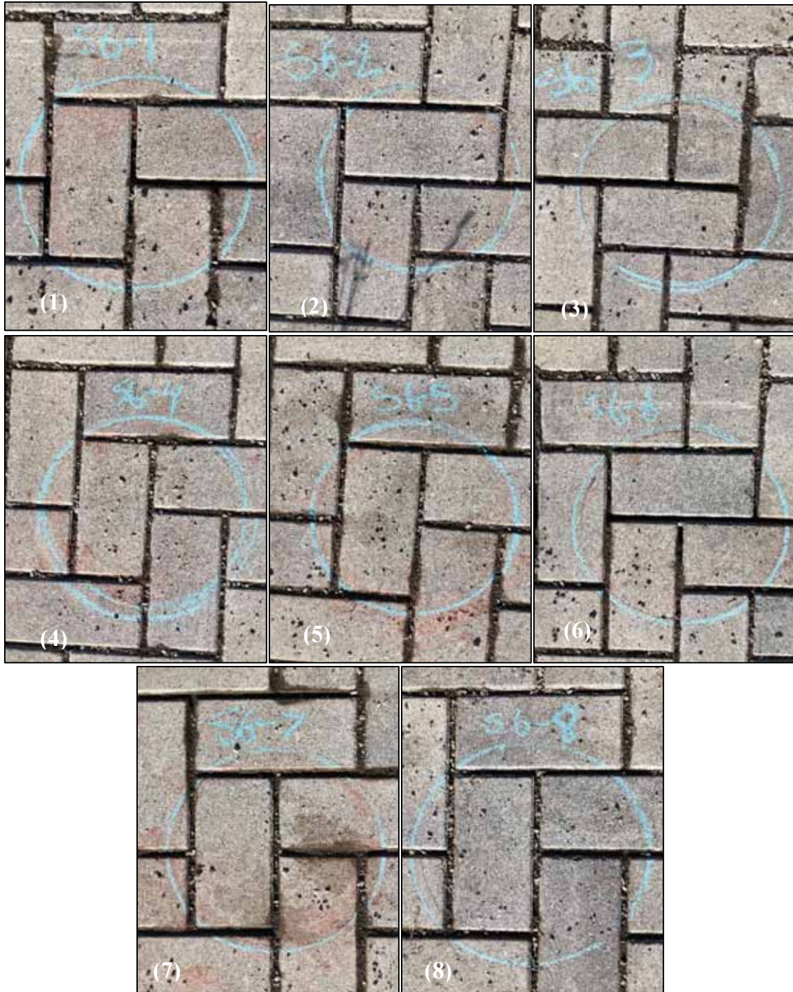
Figure J8. Post-maintenance photos of infiltration measurement locations (1-8) following a regenerative air street sweeper on Cell 6 for fourth early and repeated maintenance (TYMCO DST-6®).
