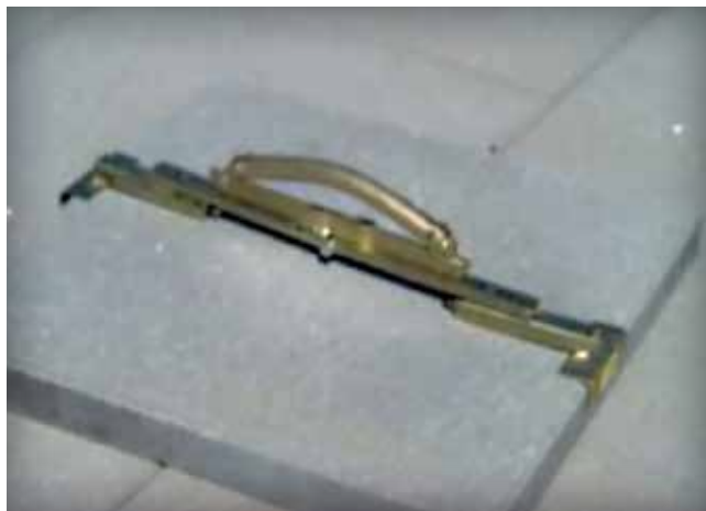
Figure 10. Single hand scissor clamp for lifting small and thin paving slabs
