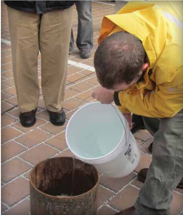
Figure 13. ASTM C1781: pouring the water into a 12 in. (300 mm) inside diameter ring set on plumber's putty.
