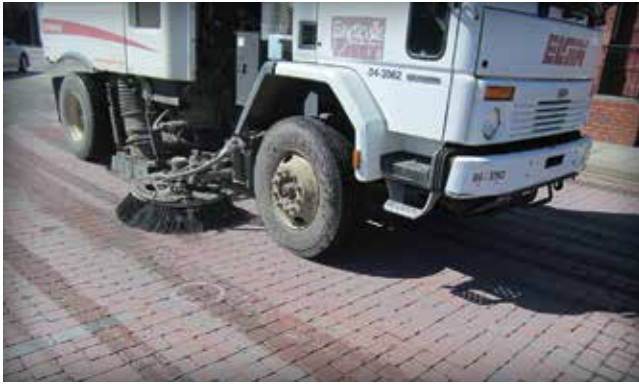
Figure 21. A regenerative air machine does routine cleaning in a PICP parking lot.
