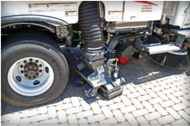
Figure 22. A true vacuum machine cleaning neglected PICP.
