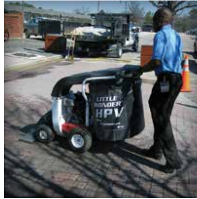
Figure 18. Walk-behind vacuum cleans a small parking area.
