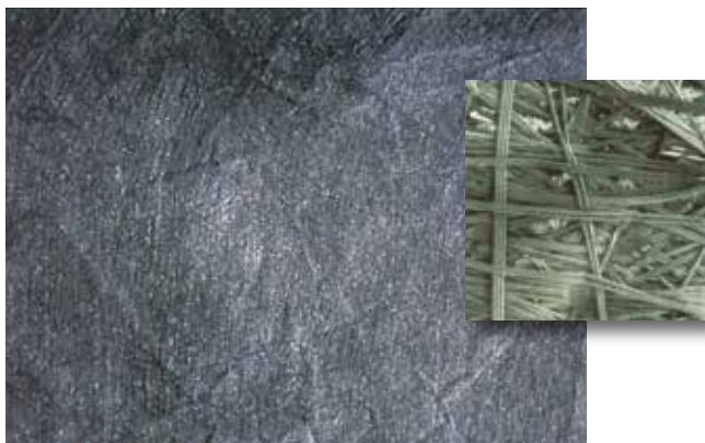
Figure 15. Non-woven heat bonded geotextile with close-up
