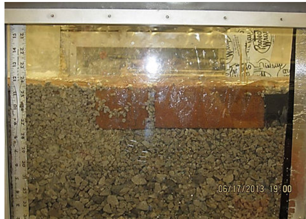
Top left and right: Flume containing PICP measures surface and subsurface flows and volumes. Bottom left and right: PICP surface at the flume end and cross section with jointing, bedding and No. 57 stone base.
