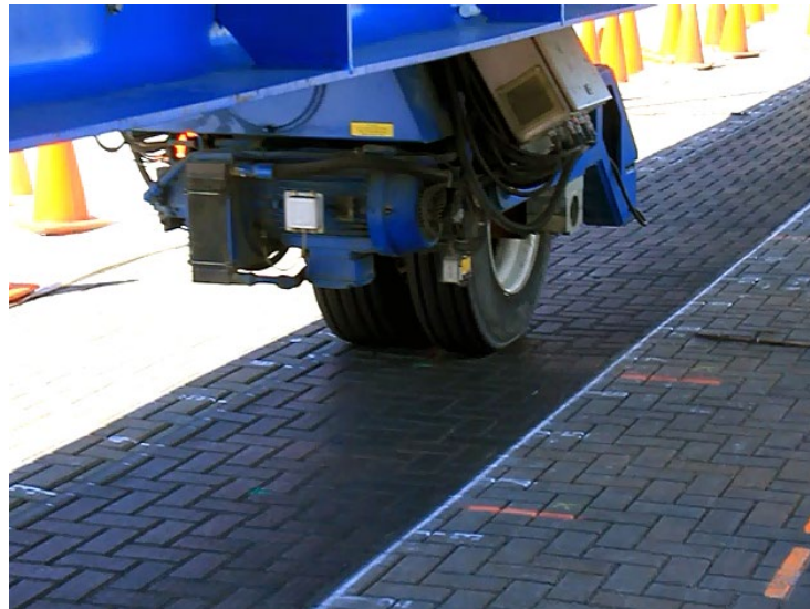
A Heavy Vehicle Similar applied up to 2.6 million ESALs on PICP section in dry and saturated conditions. The response of the pavement was used to calibrated models to determine the PICP subbase thickness.
