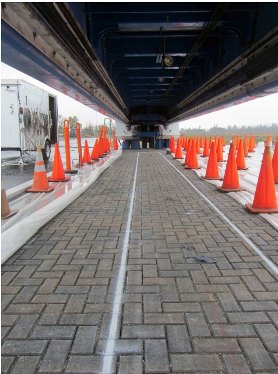
A Heavy Vehicle Similar applied up to 2.6 million ESALs on PICP section in dry and saturated conditions. The response of the pavement was used to calibrated models to determine the PICP subbase thickness.
