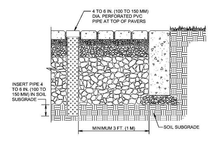
OBSERVATION WELL IN PERMEABLE INTERLOCKING CONCRETE PAVEMENT
