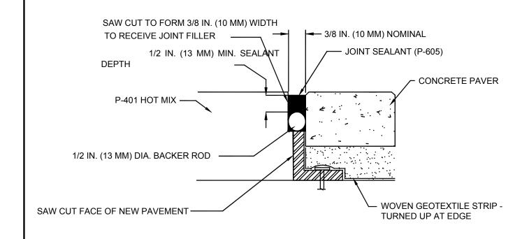
AIRFIELD PAVEMENT INLAY IN ASPHALT AT EDGE RESTRAINT
