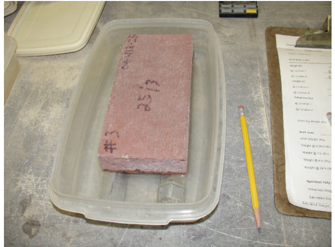
Figure 3—Specimen Undergoing the Water Uptake Test Method
