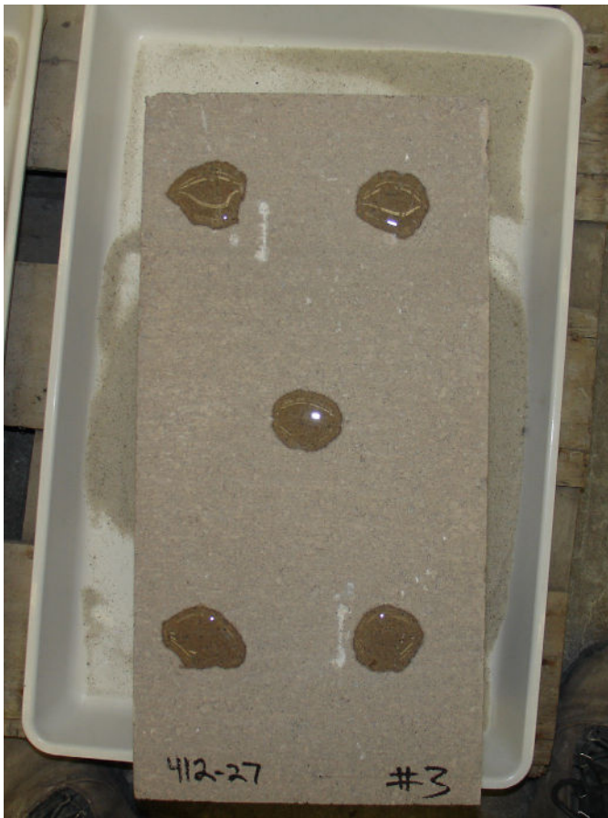
Figure 1—Specimen Undergoing the Water Droplet Test Method
