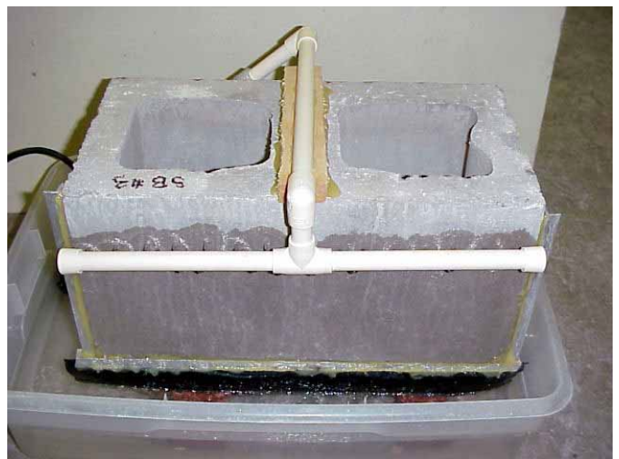
Figure 2—Specimen Undergoing the Spray Bar Test Method
