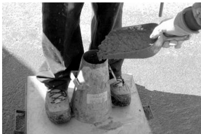
Figure 1—Filling the Slump Cone
