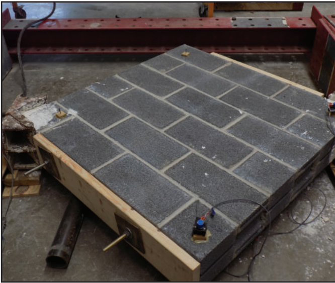
Figure 5—ASTM E 519 Racking Test Specimen
