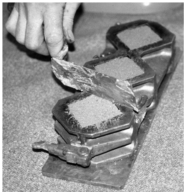
Figure 2—Striking Off Mortar Cube Specimens for Compressive Strength Testing
