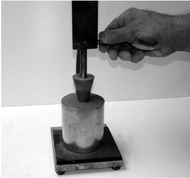
Figure 1—Mortar Consistency as Measured Using Cone Penetrometer
