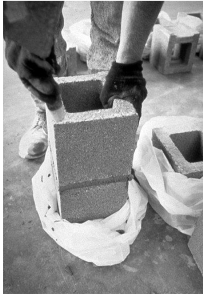
Figure 3—Constructing a Half-Length Prism in a Plastic Bag
