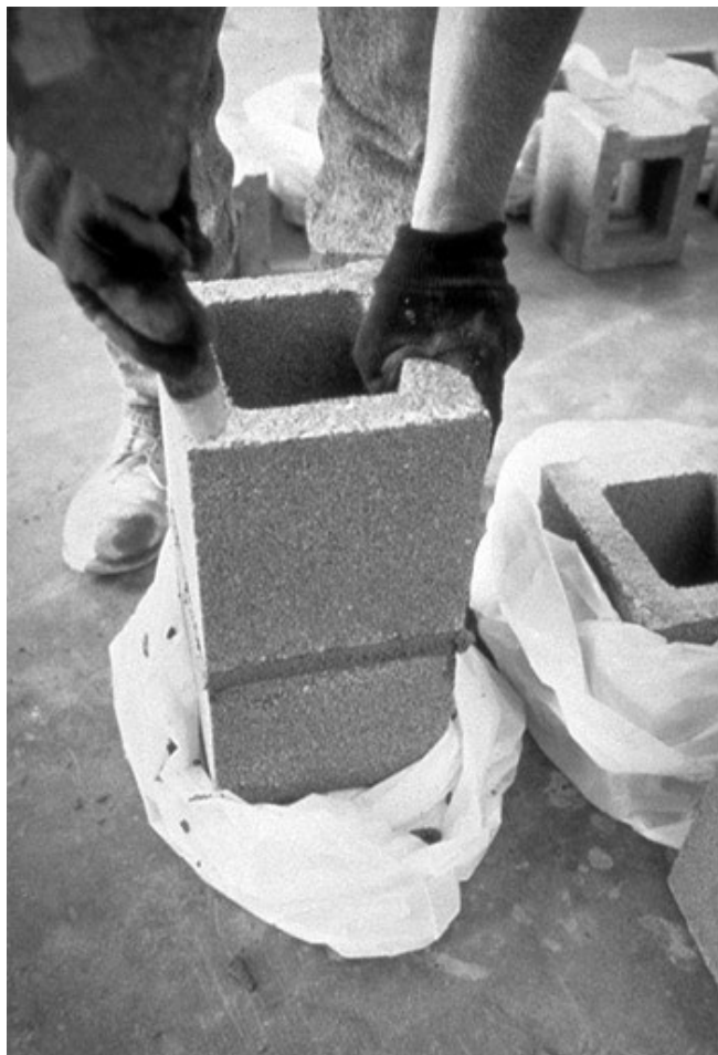
Figure 3—Constructing a Half-Length Prism in a Plastic Bag
