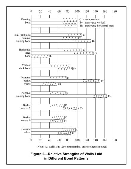
and walls built with units laid in a diagonal position were more than 50% stronger because more mortar bond area is included in the "saw-tooth" line across the wall width.
