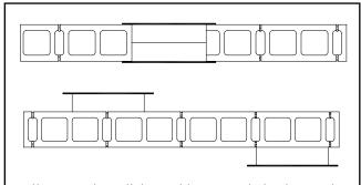
Wall-mounted medicine cabinets preclude the need to penetrate the common wall in multi-family housing. Off-setting full or partial wall penetrations also reduces noise transmission.
