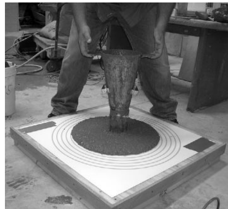
Figure 1—SCG Slump Flow Test
