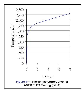
The ASTM E 119 fire test time/temperature protocol is shown in Figure 1.
