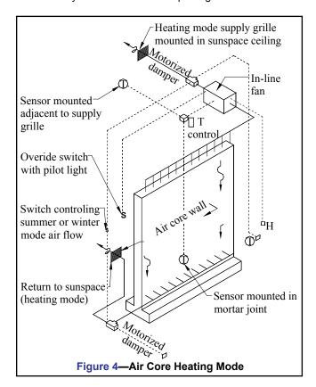
The following temperatures should be continuously monitored for improved system performance: mass, supply air, building air near the thermostat, and outdoor air.
