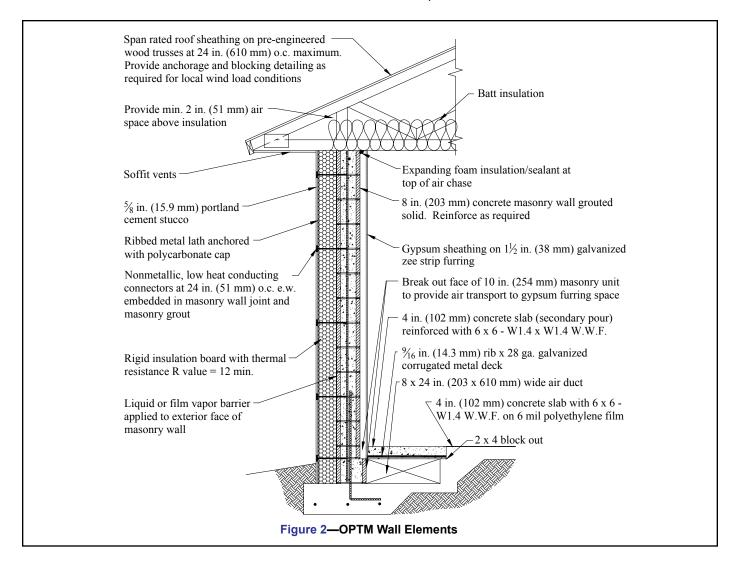
Sheet metal ducts, where used, should be properly insulated. Some codes may require fuse-link fire dampers as required in active solar air systems. These provide a good safety feature, even if their use is not mandatory. Smoke detectors can also be interfaced with hybrid fans in order to render them inoperable in the event of fire or smoke.
