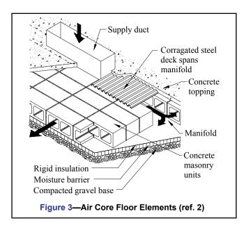
In warmer climates (lower HDD), it may be cost effective to insulate the masonry from high summer soil temperatures, improving its potential for cooling. In colder climates, the high insulation R-value not only improves air core performance, but reduces the overall building heat load.
