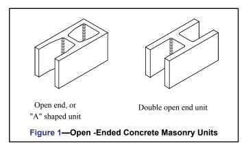
Because mortar must be placed on concrete masonry webs adjacent to grouted cores to contain the fluid grout, full mortar bedding is sometimes specified when grout is used. Mortar bedding is a design issue as well, as the section properties of a wall with face shell mortar bedding are different from those of a fully bedded wall.
