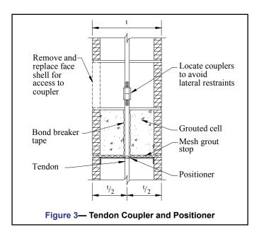
In all details, the tendons must be able to slip freely. If grout encases the tendon either totally or at restraints or bond beams, a bond breaker such as poly tape should be used to allow the tendon to slip.
