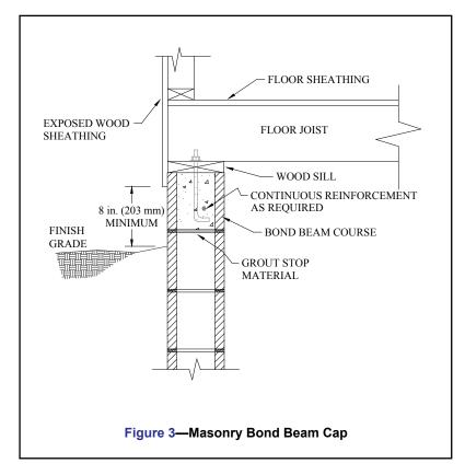
Bond beam units are specifically designed to accommodate horizontal reinforcement and grout as shown in Figure 4. Bond beam units can be either solid bottom or open bottom. The latter requires a screen grout stop or expanded metal to contain the grout within the unit. A reinforced bond beam is preferred to solid units or solid bottom units with solid head joints since the reinforcement in bond beams will hold any cracks that form tightly together to prevent termite entry through the cracks.
