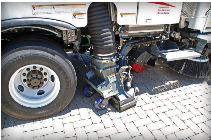
Figure 22. A true vacuum machine cleaning neglected PICP.
