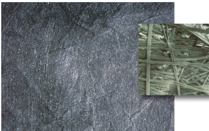
Figure 15. Non-woven heat bonded geotextile with close-up
