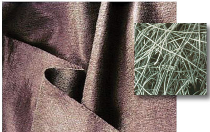
Figure 14. Non-woven needle punched geotextile with close-up
