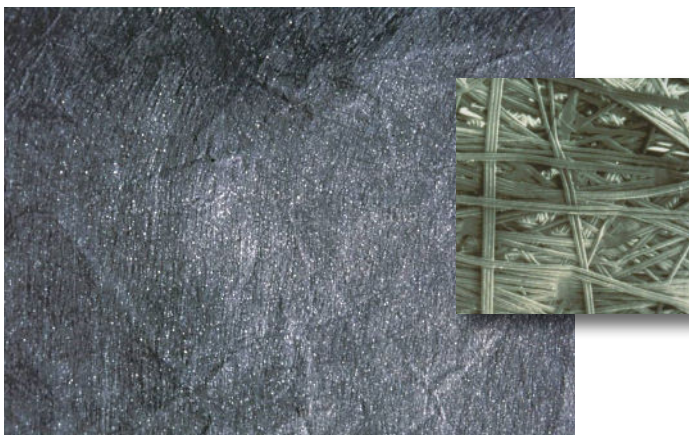
Figure 15. Non-woven heat bonded geotextile with close-up
