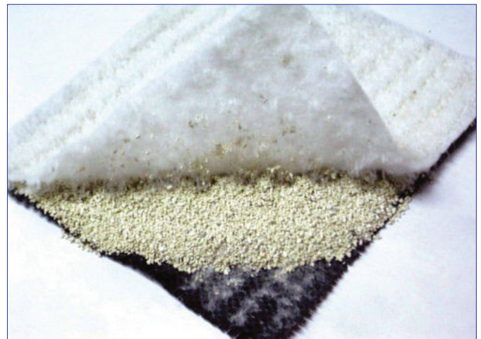
Figure 6. Geosynthetic clay liners
