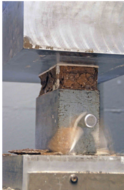
Figure 6. Left: a capped concrete paver under load in a compression testing machine; Right: a paver tested in compression; the moment it breaks is the recorded load.
