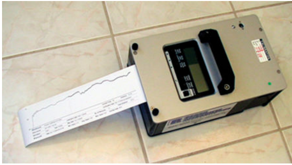
Figure 2. The BOT 3000 device measures the dynamic coefficient of friction (DCoF) and is manufactured by Regan Scientific Instruments, Inc., in Southlake, Texas. Photo credit: Jack Trumpet
