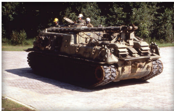
Figure 13. The completed paved area from Figure 12 receives tank traffic at the U.S. Army Proving Grounds in Aberdeen, Maryland.
