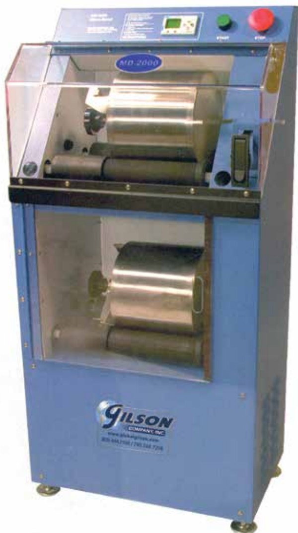
Figure 1. The Micro-Deval test apparatus. Source: Gilson Company
