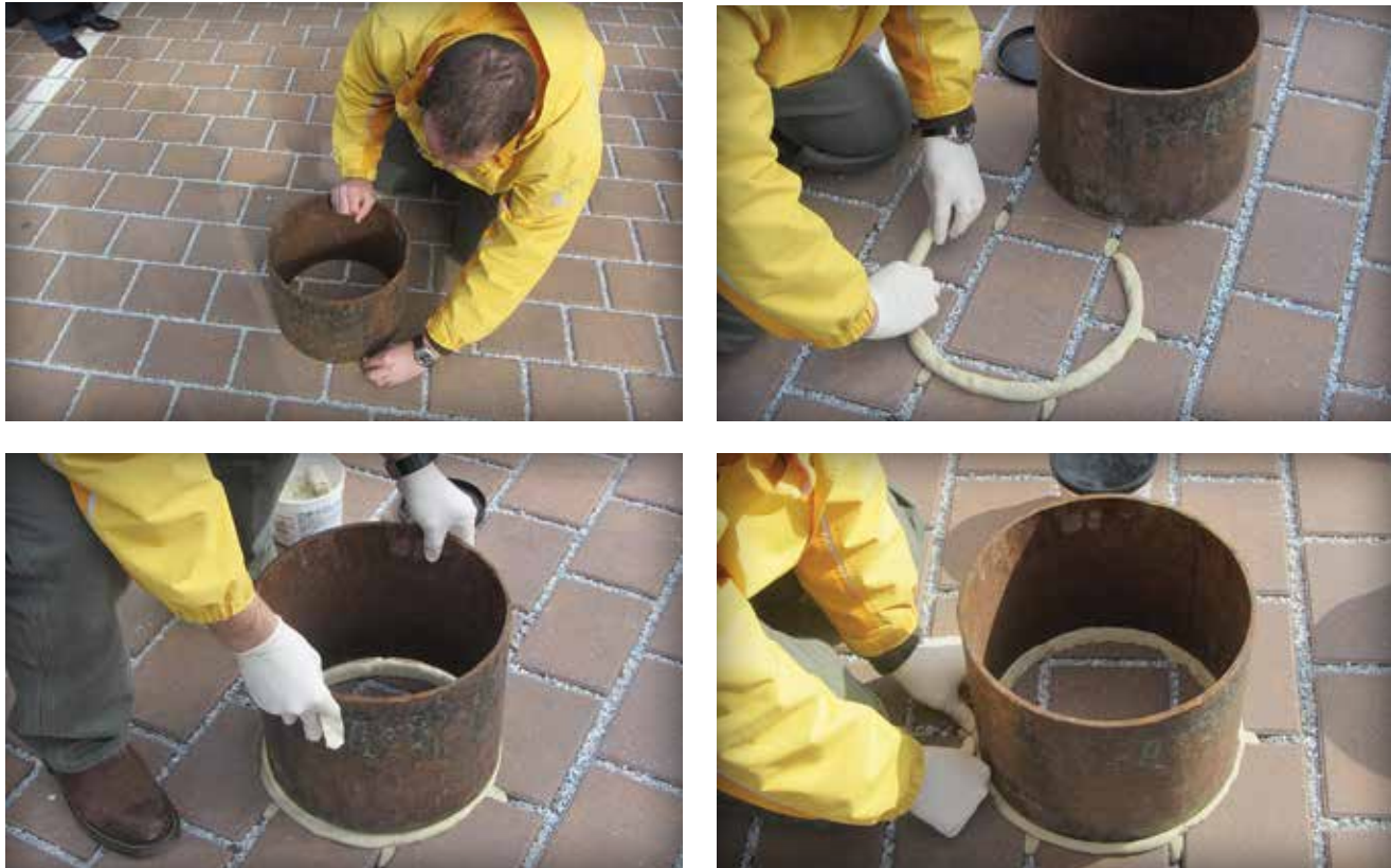
Figure 5-11. Steps in setting up test equipment for measuring surface infiltration using ASTM C1781. Left to right: Marking the location for the plumber’s putty; placing the putty on the mark; seating the ring onto the putty; and pressing the putty against the outside and inside of the ring to help create a waterproof seal.
