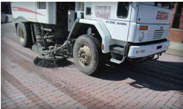
Figure 5-20. A regenerative air machine cleaning a PICP parking lot.
