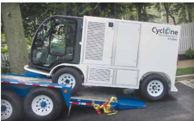
Figure 5-22. Equipment that provides combined power washing and vacuum.
