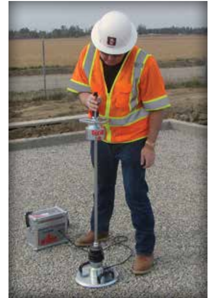
Figure 4-11. An LWD testing a compacted No. 57 base layer. This should be done on a base with a minimum 10 in. (250 mm) thick compacted subbase under it.
