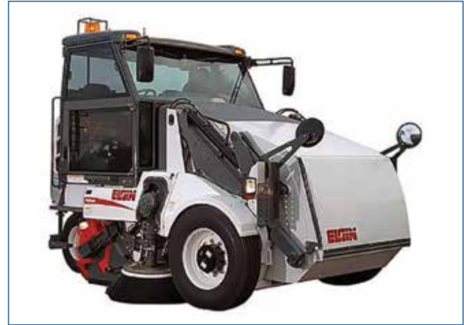
Figure 5-19. Mechanical sweepers use no vacuum, making them the least effective of large cleaning machines.
