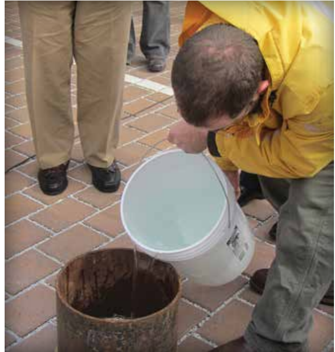
Figure 5-12. ASTM C1781: pouring the water into a 12 in. (300 mm) inside diameter ring set on plumber's putty. A maximum 0.6 in. or 15 mm deep head of water is maintained on the paver surface while pouring. Depth marks written on the inside of the ring can help establish consistency for pouring to this depth.
