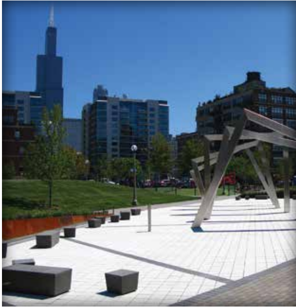
Figure 1-9. Park 542, also known as Mary Bartelme Park, located in Chicago's West Loop, includes PICP with a white titanium oxide cement to help reduce air pollutants.
