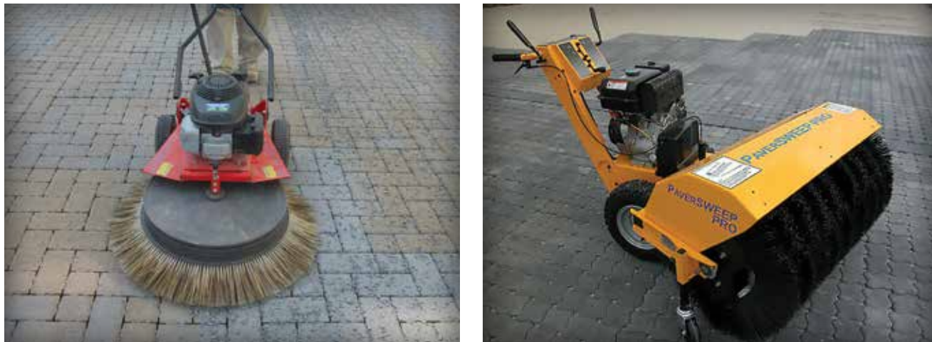
Figure 5-15. Rotary brushes increase cleaning efficiencies.
