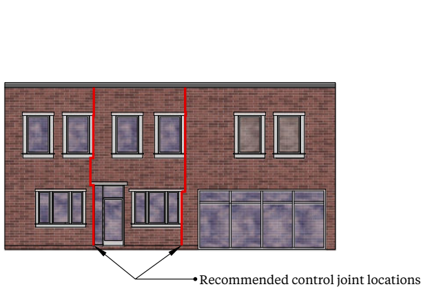
FIGURE 9—Example of Veneer Control Joint Placement
